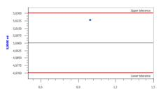
These final test values refer to the delivered nominal volume (max, volume), instrument and liquid (dist, water) at equilibrium with ambient temperature (20 °C). The test was effected according to ISO 385
