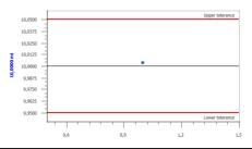
These final test values refer to the delivered nominal volume (max. volume), instrument and liquid (dist. water) at equilibrium with ambient temperature (20 °C). The test was effected according to ISO 385
